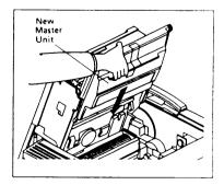
5. Push down on the bright green areas of the master unit to make sure each side is locked.
